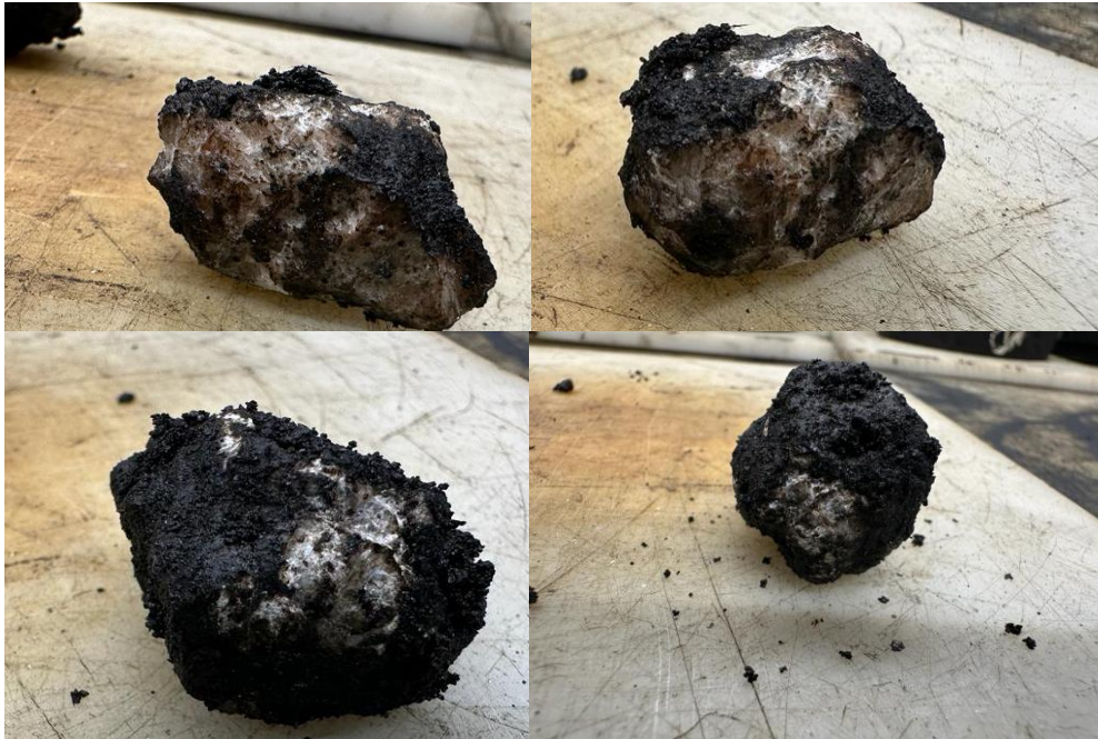
Figure 19: RB25.0C PMLC-B4 Poor Coating and Film Thickness.
